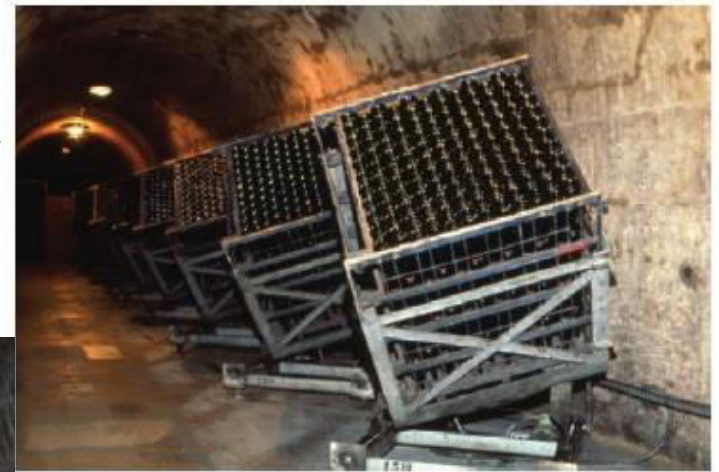
Plate 9.6 Mechanical riddling machine in Champagne. (Photo courtesy of Peper-Heidsieck, France)
